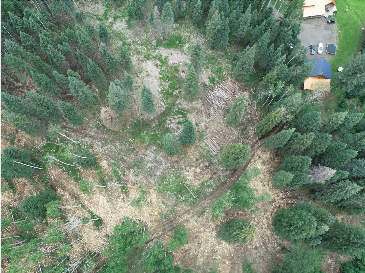
Figure 2. An example UAV image containing a view of a (red) ground control point (GCP), seen just above the dirt road near the center of this photo. Ground control points should be spaced evenly around the survey area, and ideally placed in the middle of open areas so that they are recorded in many images, and not blocked by trees.
