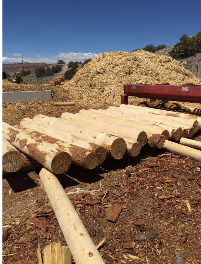
Vigas coming off the sawmill. © Carmen Austin/NMFD
